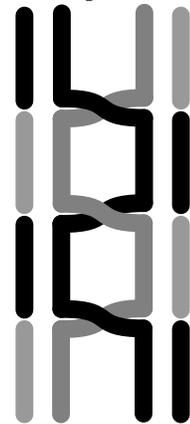
Figure 15: Inconsistently laid up stitches, left thread is sometimes behind and sometimes in front of the right thread, making the stitches lie unevenly.
